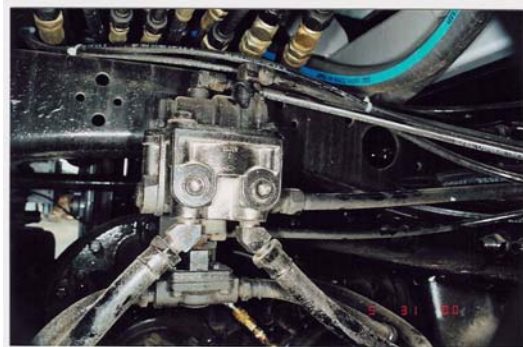
BP-R1 valve with its distinctive three-tier valve incorporated into the top of a relay valve.
